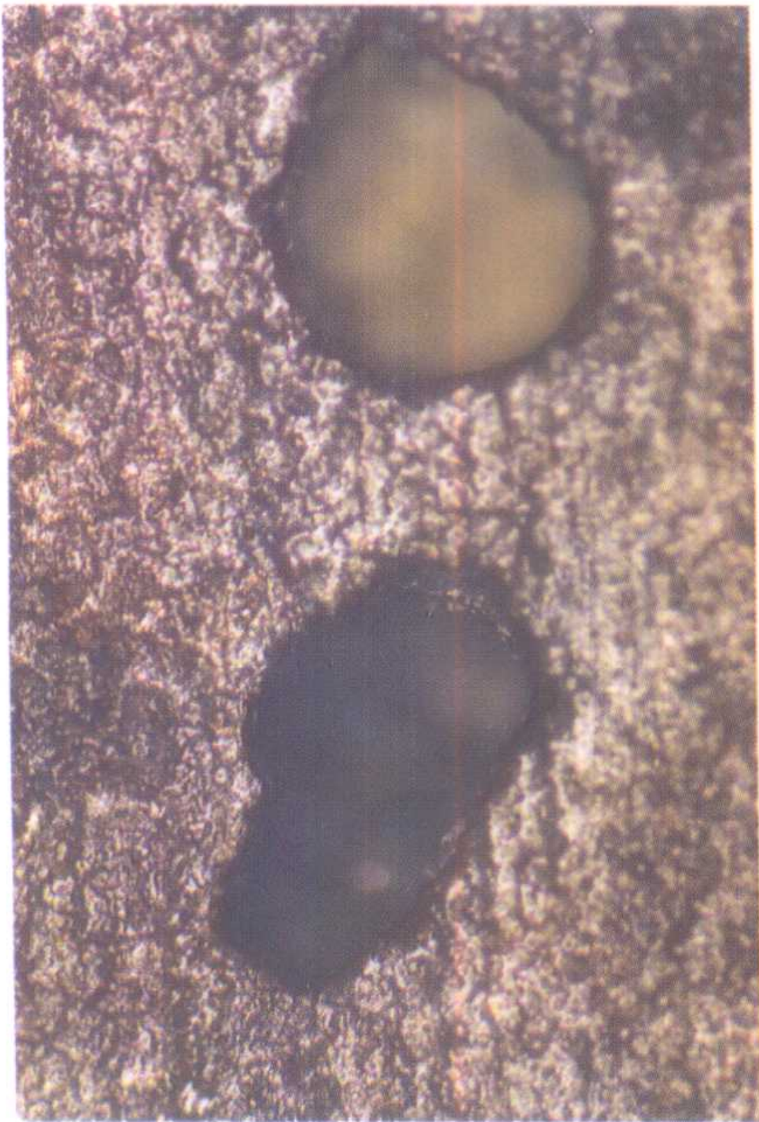
▽ 刃部上氣孔，呈長橢圓形 Oval-shaped air-holes on the blade
